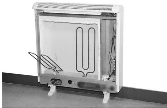
9. - Place the storage bricks carefully, with the flat side facing the back of the heater. Arrange two row levels of bricks.
