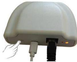
**4.2** With the hub in association mode, press
