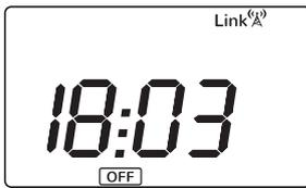
It is possible to put SSH in standby mode where the heater does not maintain any set temperature or run any programs. It keeps the time settings configured previously. When in this mode, the heater will display the current time and the icon .
