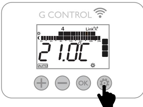
It is possible to modify the general settings. During any operation mode, press & release , the display shows the flashing temperature symbol and the RF symbol .
