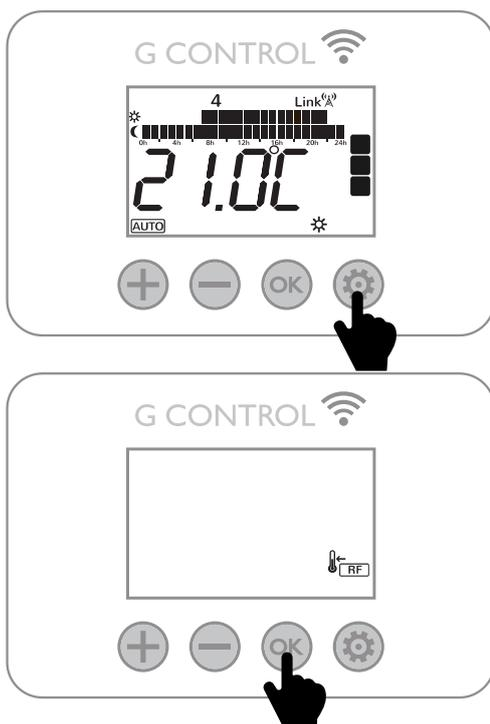
To modify the set temperatures within the program permanently, press and release
