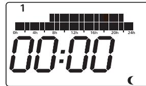
The first segment will start to flash. By pressing you can select whether you want a Frost Protection setting (3°C), Moon setting (18°C) or Comfort setting (21°C). Now press to move to the next 1 hour time interval.
