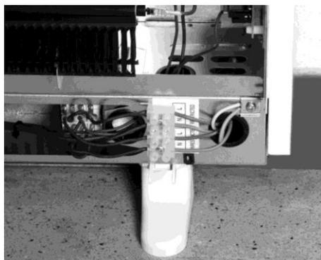
7. - Disconnect the aluminum heating element by removing the FAST-ON terminal on each end of the element.
