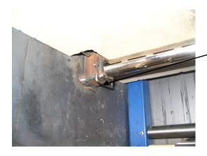
Remove retaining clip by lifting out and sliding back
