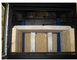
Sit baffle plate on top of firebricks as shown. Ensure there is no creosote/soot accumulated on top side of baffle and at the base of the flue spigot.
