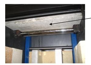
Baffle correctly in place. Air tube secured by retaining pin at left hand side.
