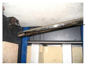
With one hand, support weight of baffle. With the other hand, slide air bar to the right, then across to the left to remove entirely.
